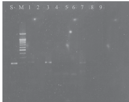
Figure 2. PCR amplification of grouper code GP5 using primers specific to RSIV showed a product at ~187 bp of sample number 1, 3 and 7. (M = 100 bp Ladder marker; S = sea bass iridovirus positive control)
